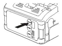
2. Reach under the printer and unlatch the battery compartment cover.
